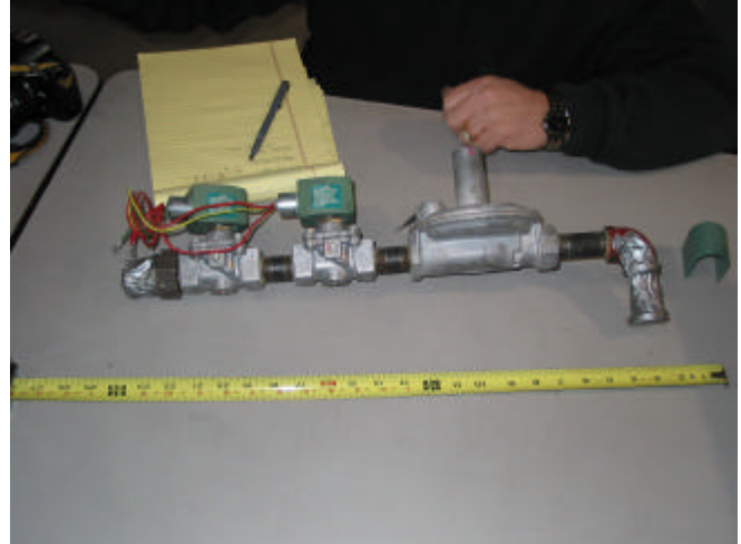
Pilot Gas-Control Valve Train
